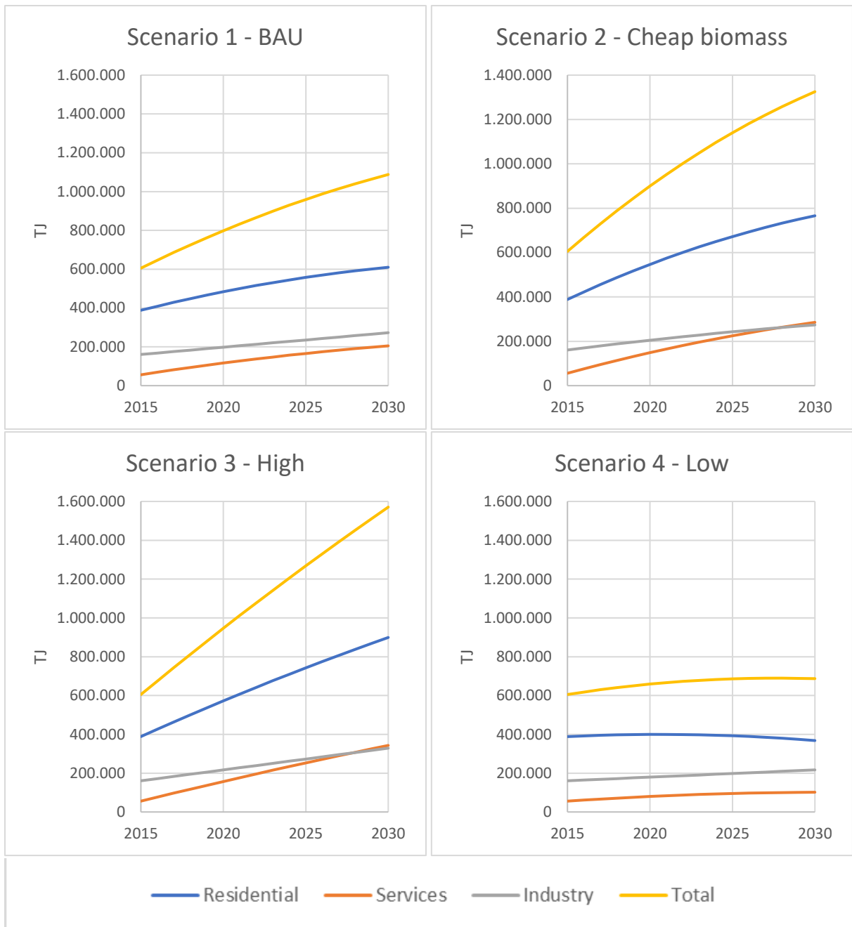
Figure 19 – Total NW-EU solid biofuel demand for small scale heat, 2015-2030 for the 4 scenarios (in TJ)
