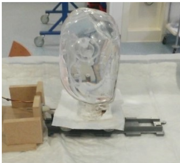
Figure 4.11: The setup for translational motion consisted of a stepper motor that drives the motion of the phantom. The stepper motor was connected to an Arduino and was programmed to perform a sinusoidal motion.
