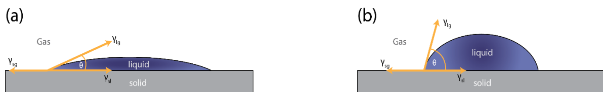
Figure 24. (a) A liquid which wets the surface well creates a small solid-liquid contact angle. (b) A liquid which does not like to wet the surface creates a large solid-liquid contact angle.
