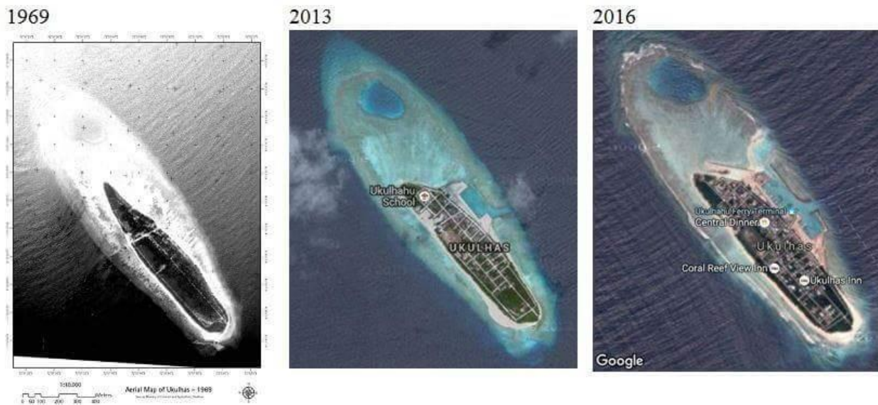
Figure 2-1: Three images of the island of Ukulhas, which shows the increase in beach erosion, due to harbor construction 6
