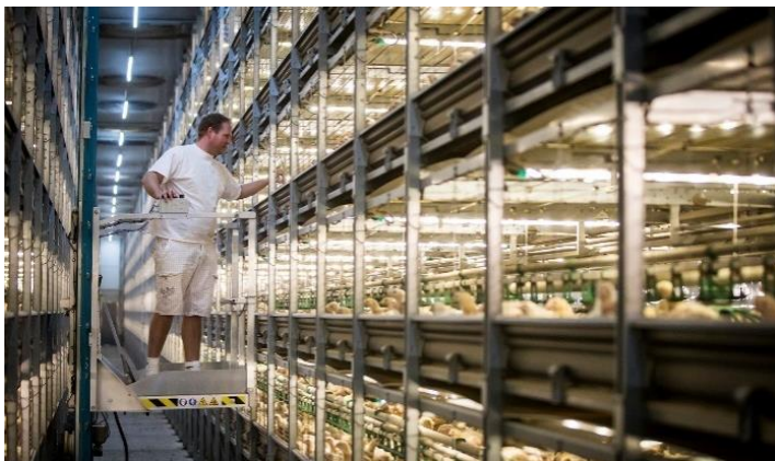
Figure 2: One compartment consists of two rows of six Patio units (levels) on top of each other
