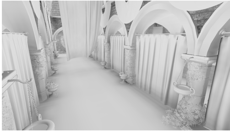
Figure 3.31: Ambient occlusion using Voxel Cone Tracing. The image was created using the engine written for this research.
