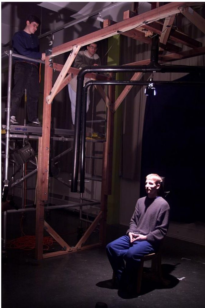
Fig. 5. The face-scanning light stage used by Debevec et al. [7] consists of two-axis rotation system and a directional light source. The outer black bar is rotated about the central vertical axis and the inner bar is lowered one step for each outer black bar's rotation. Video cameras outside the stage record the facial appearance. The inset shows a long-exposure photograph of the light stage in operation.
