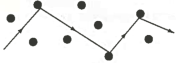
Figure 4: the Drude model. The path an electron might follow in a metal. In between the ions, the electron moves in a straight line. On the ions the electron scatters randomly. Reprinted from Reference [9].
