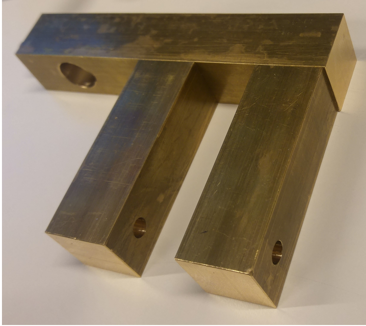
Figure 3.3: Designed holder for the LED and photodiode
