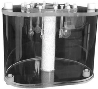
Figure 6: The NEMA 2012/IEC 2008 phantom, similar to the NEMA 2007 phantom. The phantom is torso-shaped. It contains six spheres and a background compartment that can be separately filled. Retrieved on 07/12/16 from the website of Biodex: http://www.biodex.com/nuclear-medicine/products/pet-positron-emission-tomography/pet-phantoms/pet-phantom-nema-2012iec-200 .
