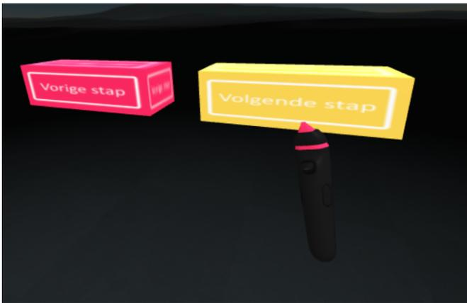
Fig. 4. The 'previous step' and 'next step' buttons. They turn yellow when the controller is close enough to select them.
