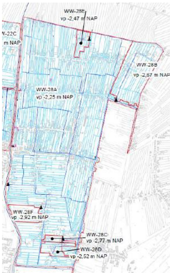
Figure 2.2 - schematization of the Gouwepolder surface water level system: Gouwepolder (28A), Spoelwijk (28B), Berkenbroek-Noord (28C), Berkenbroek-Zuid (28D), Koetsveld (28E) and Gouwedreef-Randenburg (28F) (HHR, 2017)
