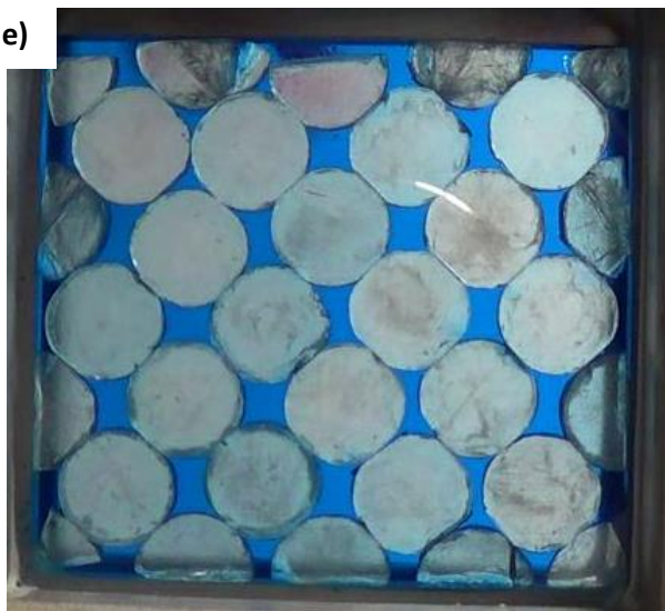
Figure 30. The five different type of experiments at a stress of 4.0 MPa. What can be seen is that in none of the experiments the discs that aren't in contact with the steel have failed. However, a difference can be seen in the outer discs: where in the hexagonal experiments (a and b) maximum one semi-circular disc has failed, in the cubic experiments (c, d and e) multiple (semi-circular) discs have failed.
