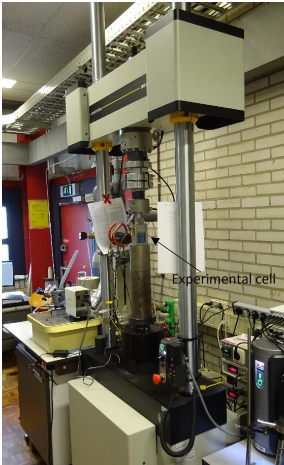
Figure 2. A picture of the experimental setup. The experimental cell is placed in the frame of the Instron and the sample is compressed by the upwards movement of the base of the machine.
