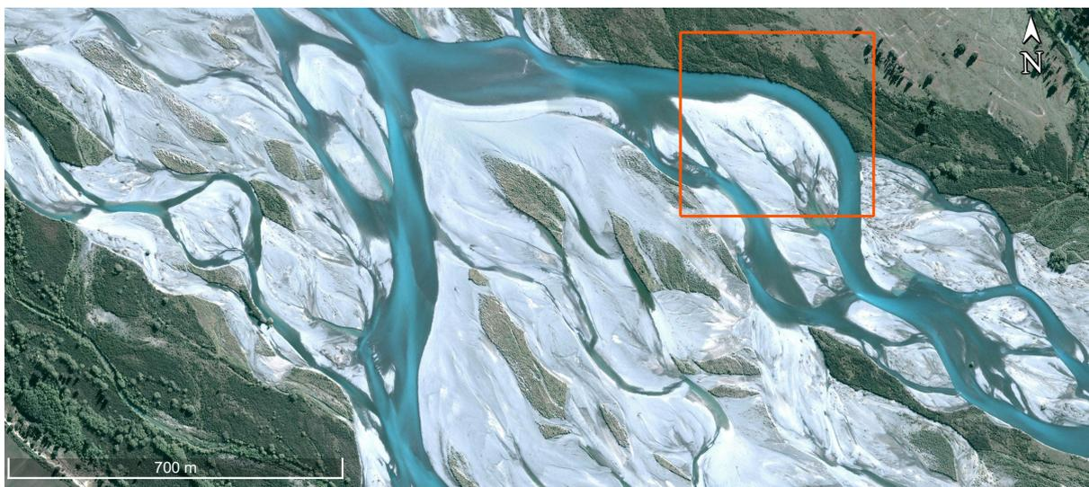
Figure 5.4: Fairly sharp river bend in braided river network, Rakaia River (NZ). Flow is from top to bottom. Distinct sorting may develop in the lower-right corner of the contoured section based on the sinuosity. Though, since this is a gravel bed river, grains are generally only mobile for bankfull or larger discharges. Consequently, bend sorting will be poorly developed, also due to unbending of flow. (Google Earth imagery, accessed January 2017)
