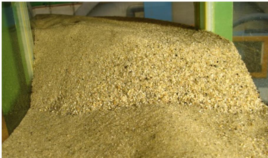
Figure 4.6: Well developed bend sorting at lee side of a dune for a steep transverse slope (exp. 22). View is upstream directed. Photo was taken unintentionally at a slight angle, so transverse slope may seem gentler than 0.22.
