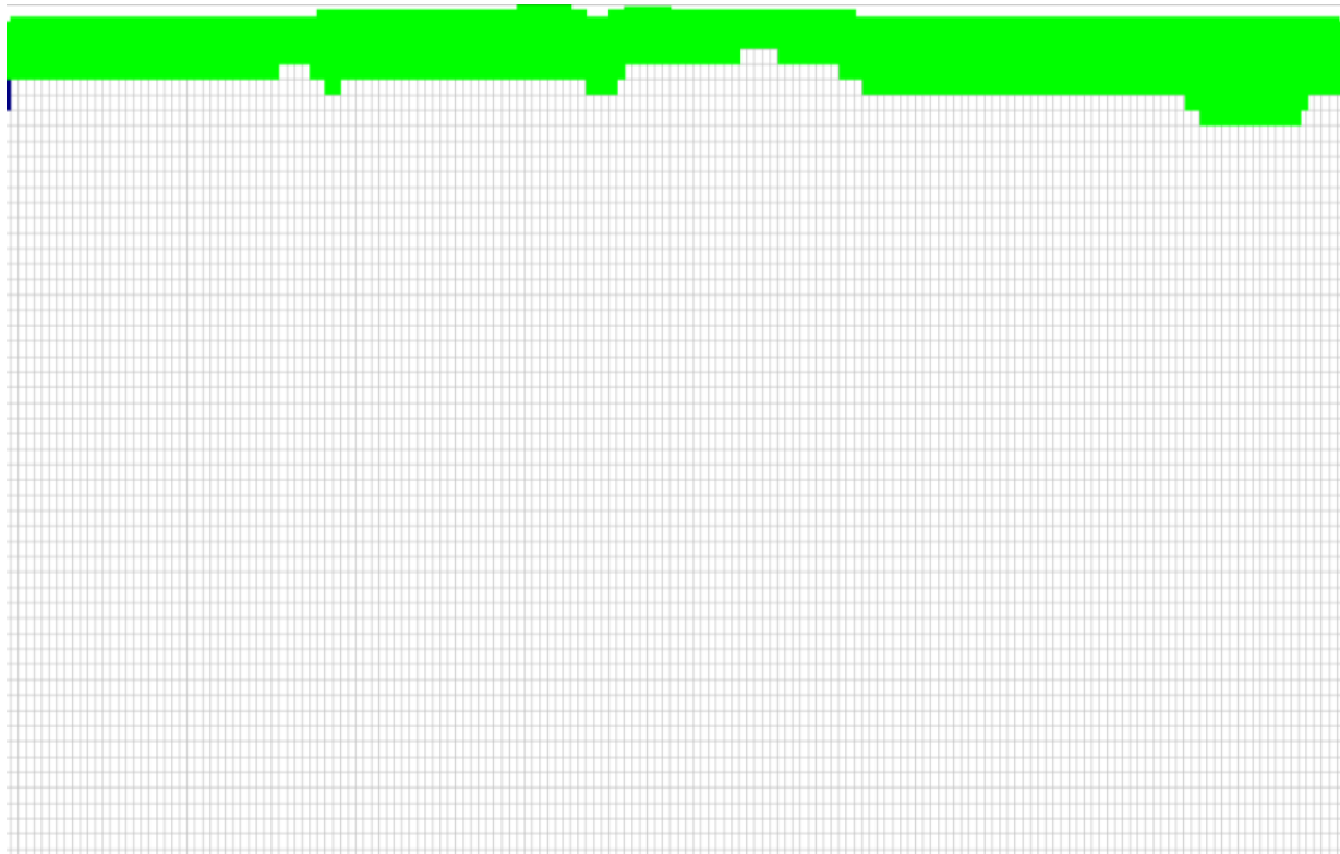
Figure 2.5: Layout of the model, 175 by 55 cells, top layer elevation and confining clay layer (green).
