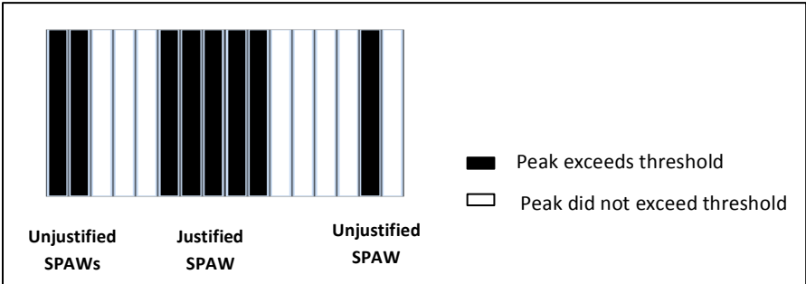
Figure 18 Schematic presentation of the final heuristic measure. In white the cross sections in which no SPAW was recognized and in black the sections in which a SPAW was recognized. With 5 or more subsequent recognized SPAWs the individual SPAWs are assumed true.
