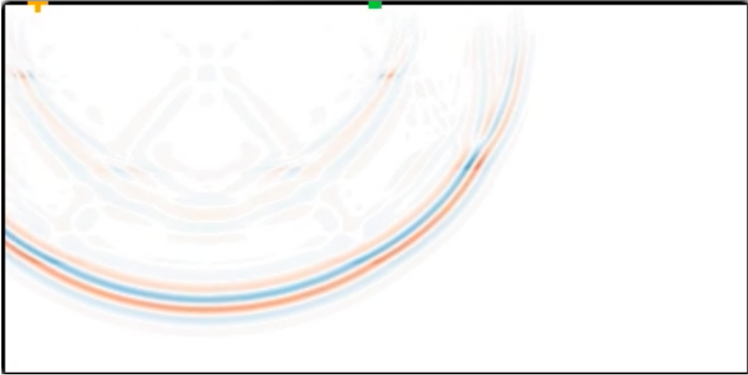
Figure 10: Two dimensional Frechet sensitivity kernels using optimal operators for the wave equation
