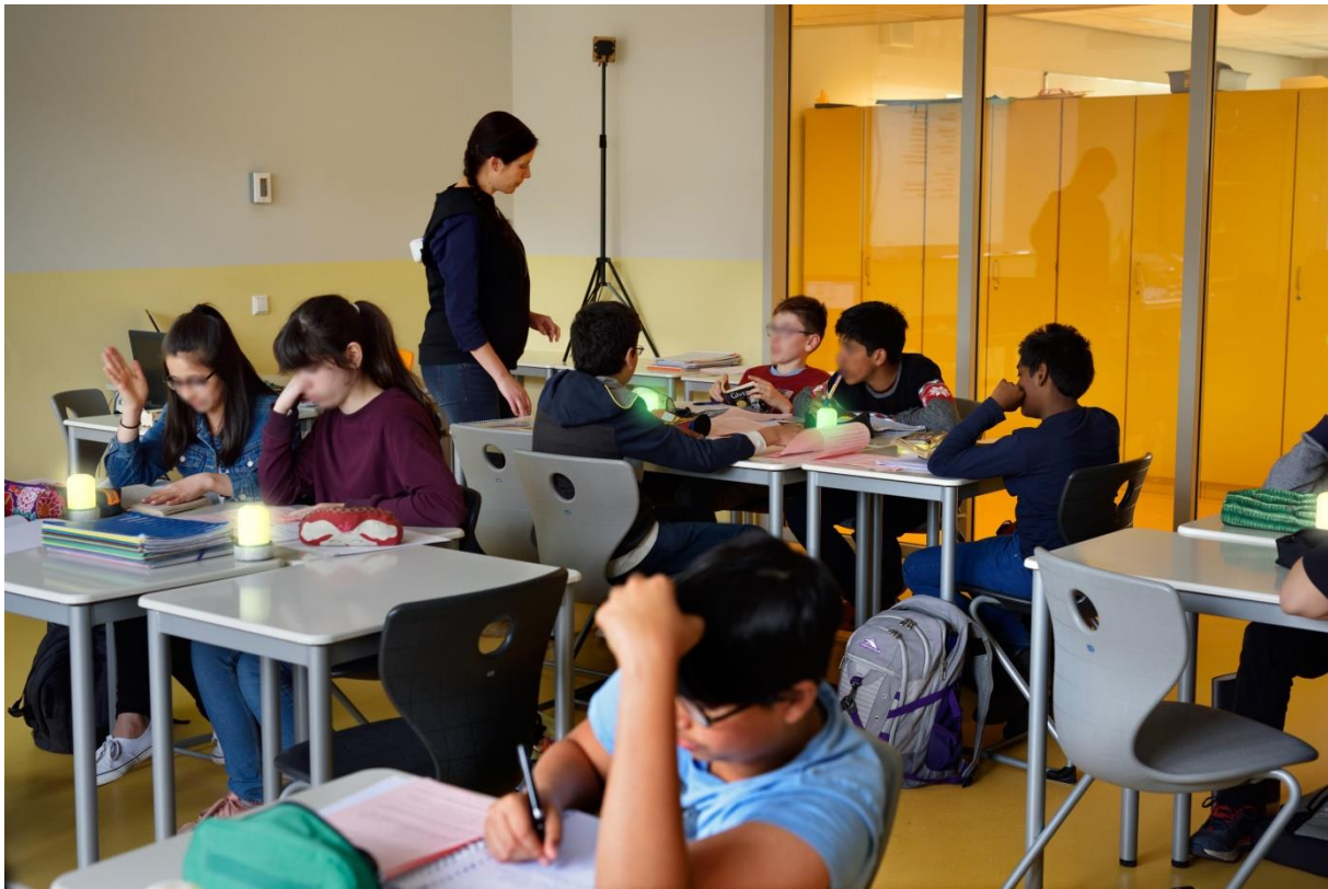
Figure 1. The FireFlies V2 system deployed in a secondary school classroom in Eindhoven. The teacher is wearing the tracking device and the lighting objects are placed throughout the classroom.
