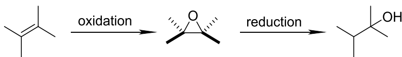
Scheme 30: Functionalization of an olefin double bond by oxidation and reduction via an epoxide intermediate product.
