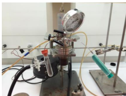
Figure 13: Mixture injection into the autoclave set up by N 2 /H 2 counter flow. A Schlenk flask under N 2 atmosphere contains the mixture. Inside the autoclave a H 2 atmosphere is present which is released while connecting the Schlenk flask to the autoclave (tube through septum). By suction with a syringe the mixture is transferred into the autoclave.
