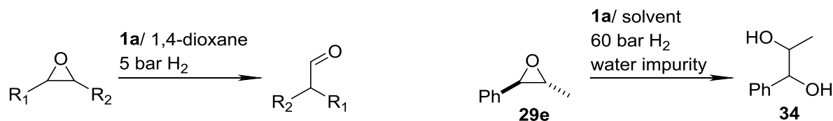
Scheme 60: Exposure of various epoxides to the FLP 1a /1,4-dioxane resulted in 1a mediated isomerization to aldehydes (left). 1a catalyzed the hydrolysis of 29e in different solvents (right).
