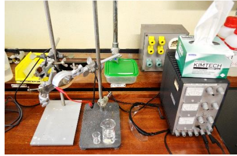
Figure 2.2. The two ring stands, stainless steel plate and power supply of the ECE set-up.
