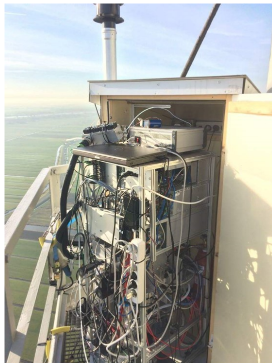
(b) Setup is removed from the insulating box for maintenance. Boundary layer is expected to be well mixed.
