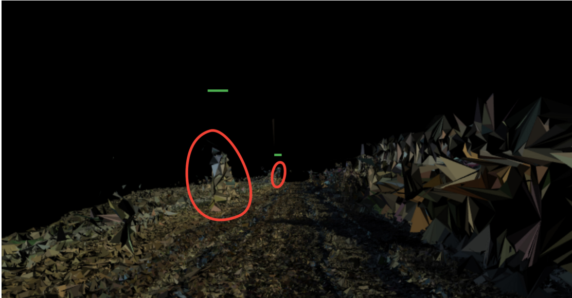
FIGURE 6.10: CCs in the baseline mesh highlighted in red. The green lines indicate their actual height. The portions above the railway are also mostly missing.
