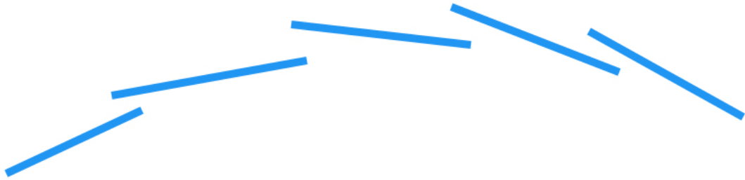
FIGURE 6.11: A schematic example of an issue that may occur if the orientation of the train or camera is incorrect. The blue lines resemble the railway tracks reconstructed from multiple frames. In this case, the orientation of the train lags behind its actual orientation, affecting the orientation of the tracks and causing a zig-zag pattern.
