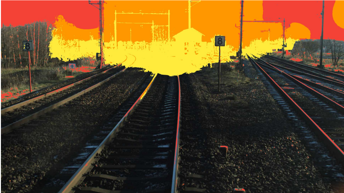
FIGURE 4.3: A visualization of the pixels that are filtered out by the optical flow threshold (yellow), brightness threshold (red) or both (orange).
