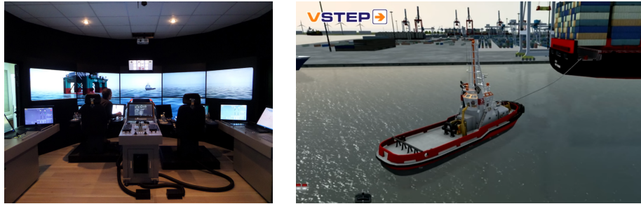
Figure 1: One of the possible NAUTIS training station from VSTEP (here for oil tankers) and a screenshot of the NAUTIS software during a tugboat training.
