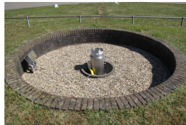
Figure 2.5: An automatic rain gauge of the KNMI in English setting (Brandsma, 2014).
