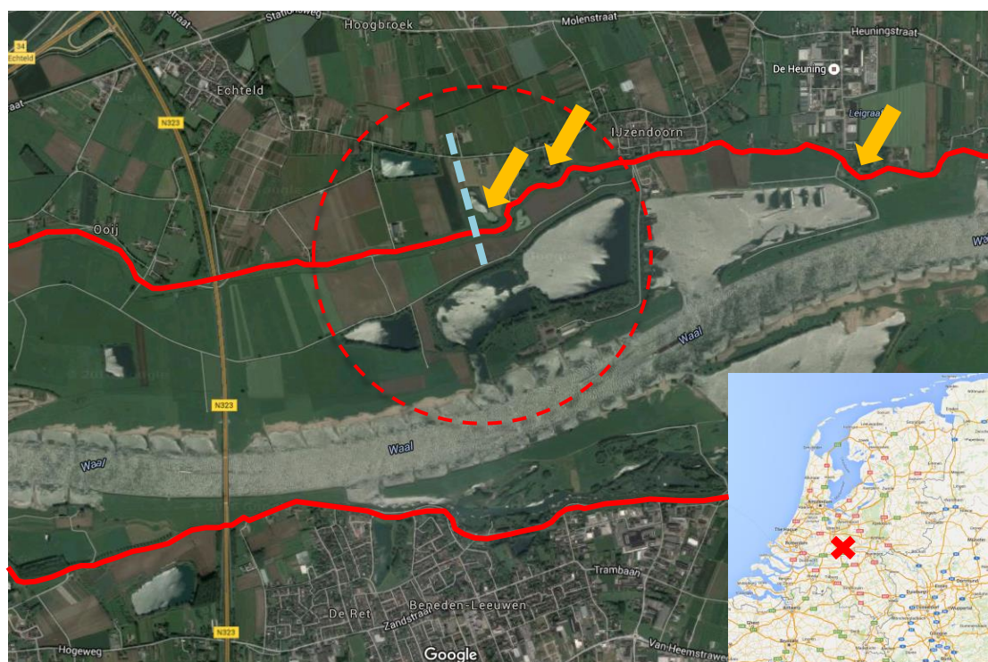
Figure 2.1 An overview of the research area. Previous research is carried out within the area indicated by red dashed circle [Koopmans and Van den Berg, 2015]. Red lines are the primary dikes, orange arrow are the locations of dike failures from the past. The dashed blue line shows the location of the lithological cross section.
