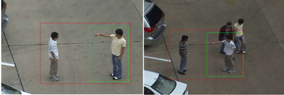
Figure 5.18: Spatial detection of interacting people. The green bounding boxes are the ground truth, while the reds are the detection results. For the interactions with class label "3" ("Pointing"), only one person is annotated in the ground truth, while both interacting people are annotated by our detector.
