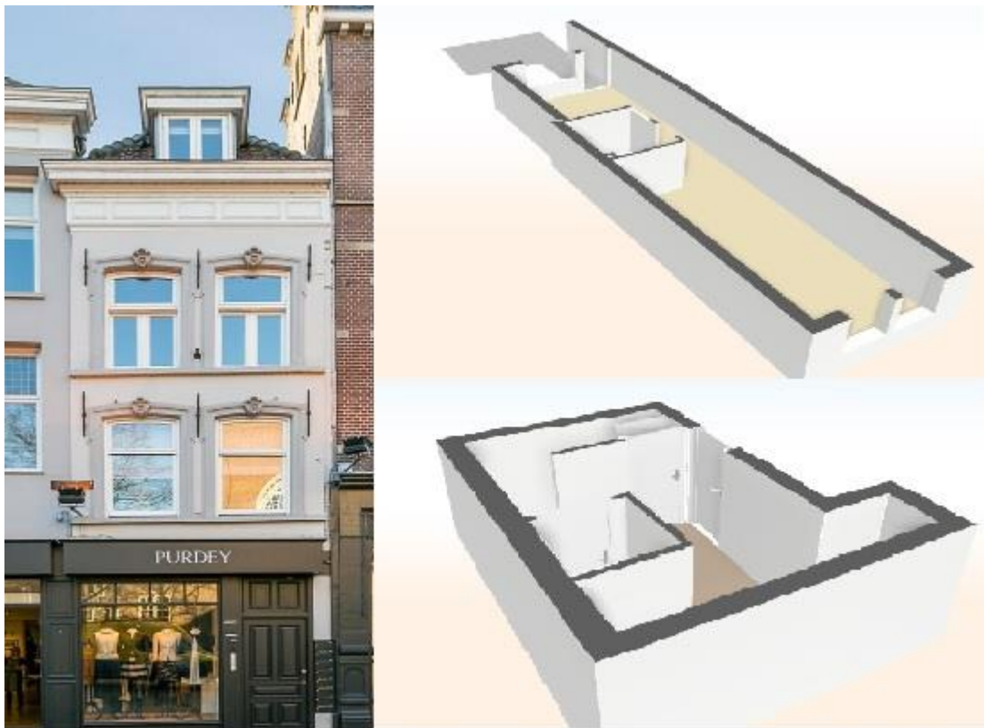
Figure 26 An apartment created within an existing building with different-shaped spaces spread over a number of floors – the top right hand picture shows the first floor and the bottom right hand the ground floor. Funda.nl
