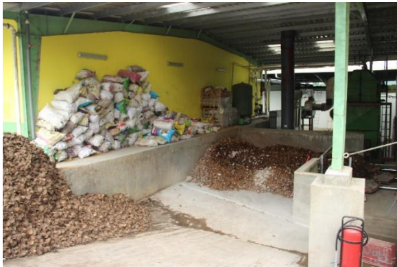
Organic waste from coconut processing is used to heat the fruit drying facilities
