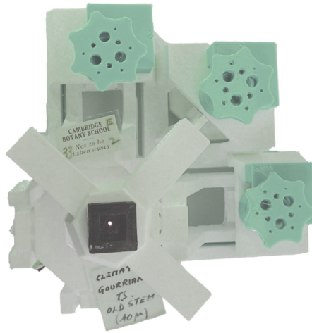
Figure 2: Photograph of the iGEM OpenScope. The three big gears control lateral motion and focus respectively the outer and center gears. The lens and camera sensor are above the sample as in traditional microscopy. A LED illuminates the sample from below. The OpenScope can mount a filter between lens and sensor to do fluorescence measurement.
