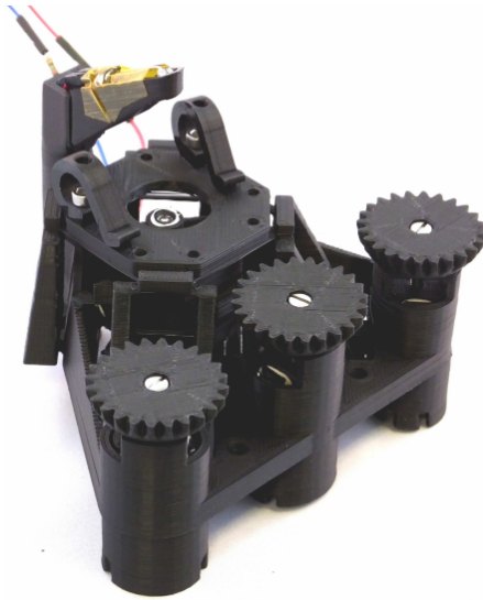
Figure 1: Photograph of the one-piece 3D printed microscope. The three big gears control lateral motion and focus respectively the outer and center gears. The sample is held by the printed clips, a white LED is mounted on a printed arm at the top and the lens from the Raspberry Pi camera module is visible though the hole in the sample stage. The camera sensor mounts underneath the microscope.
