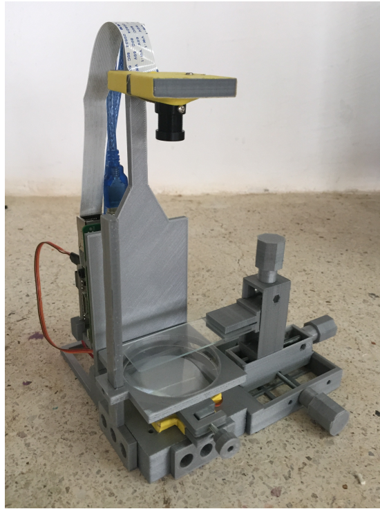
Figure 3: The FlyPi microscope. It is cheap and its possibilities are a growing. These possibilities include fluorescence measurement and more.
