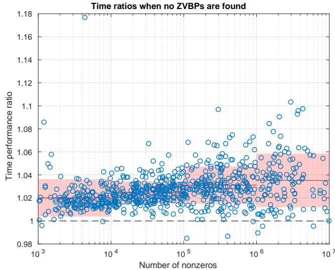
Figure 11: Ratio of running times when no ZVBPs are found, for the case P = 16 and \epsilon = 0.03 , averaged over 5 runs. Numeric values for the means are given in Table 2.
