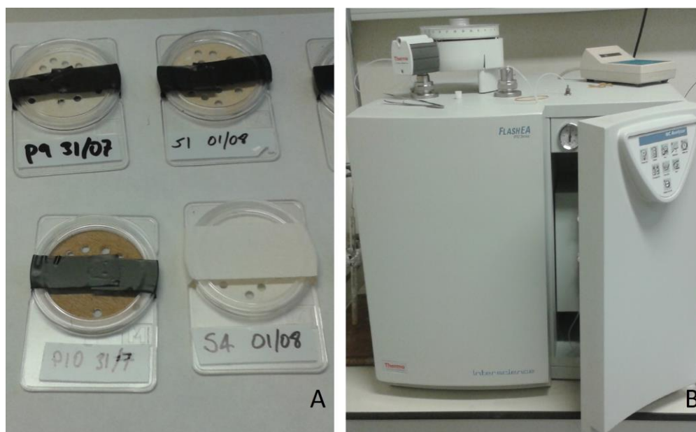
Figure 6. A) Example of punched filters, notice the difference in colour of the different filters. B) The Thermo Flash elemental analyzer 1112 series.
