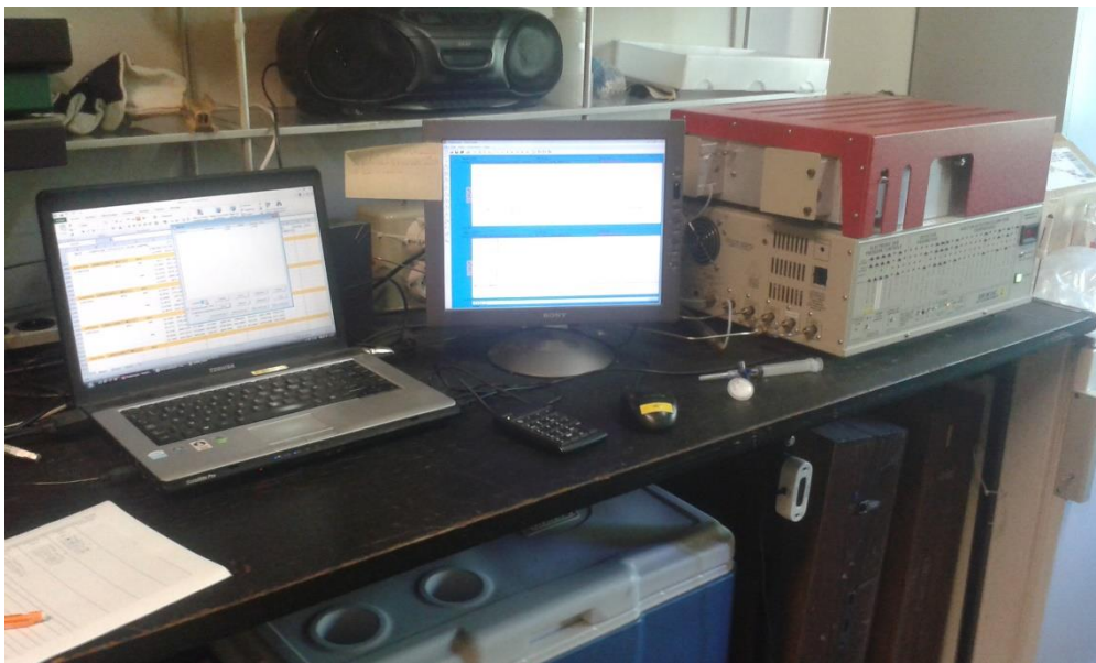
Figure 5. Setup of the dissolved gas concentration measurements in Liège, Belgium. The box with the red top is the flame ionization detector.
