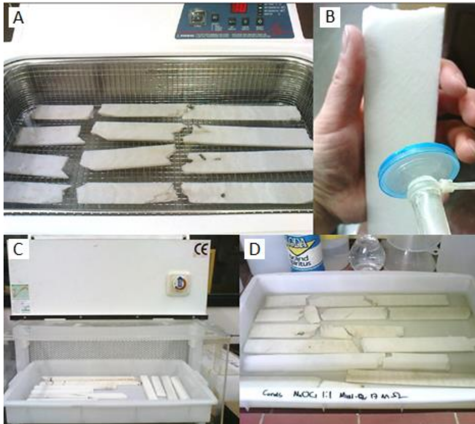
Figure 6. Coral cores treatment with: A) Coral slabs rinsed in an ultrasonic bath. B) Cleaning of the coral slab with compressed air. C) Coral slabs dried under a laminar flow hood. D) Bleaching of the coral slabs. Photographs modified after Pascher (2012).
