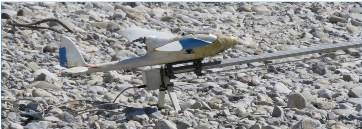
Figure 2.2 Side-view from the in 2015 used fixed-wing UAV connected with the launch platform.
