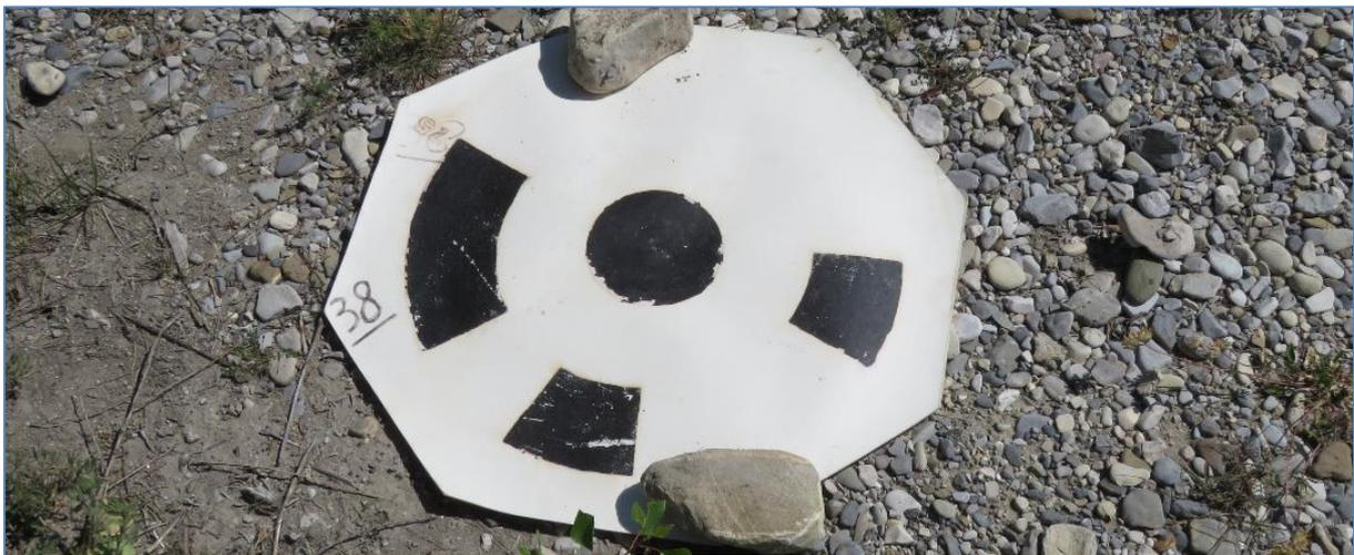
Figure 2.5 Example of a marker (number 38) used in the field.
