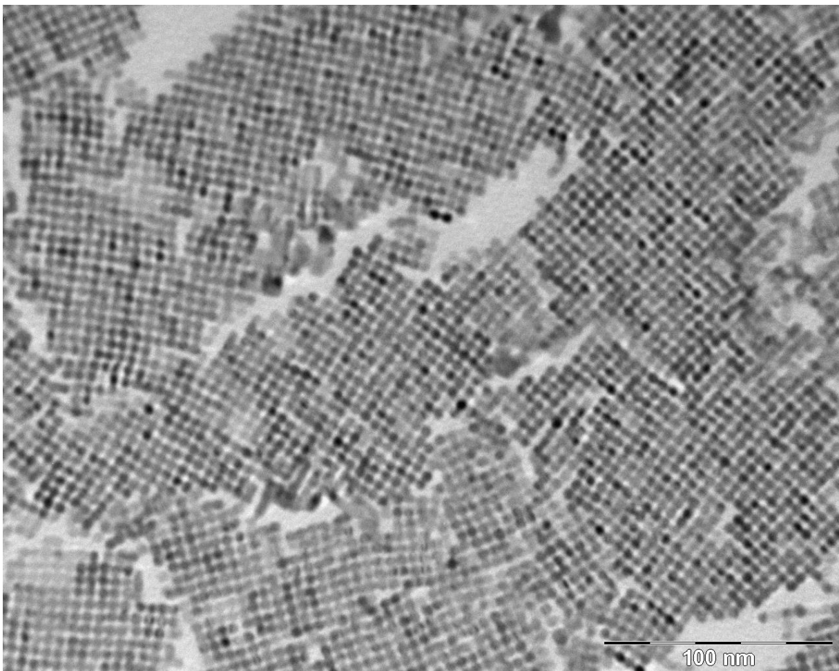
Figure 10. TEM image of square superlattices synthesized using MCT04W diluted 200 times. Multiple patches of square superlattices are shown, with a size in the order of 100-200nm. The particles aren't completely attached there is a neck in between the particles.
