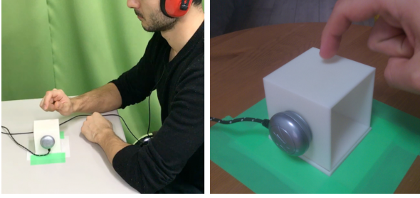
Figure 2: Setup for experiment 1: (left) Participants tap the top of a solid or hollow cube. There is visually no distinction between the two thicknesses (the opening in the right figure is faced down). The cube is placed in a holder that is firmly attached to a table surface. A piezoelectric sensor is attached to the side of the cube (right) to capture vibrations in the material.
