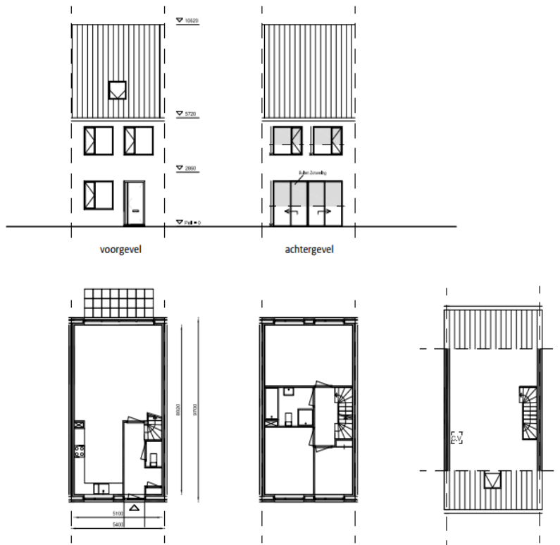
Figure 2.7: Average Dutch mid-terraced home; front façade, rear, first-, second-, and third floor (Agentschap NL, 2013)
