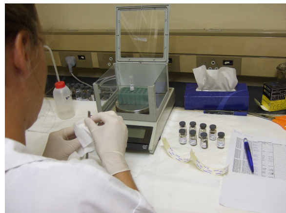
Figure 5 – Pulverization of freeze-dried material (above) and weighing of material (below) in the process of fecal extraction.
