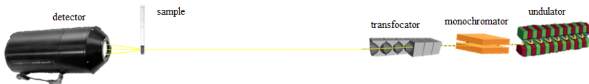
Figure 3.3: Illustration of the SAXS set-up. Images adapted from [49], [50] and [51].
