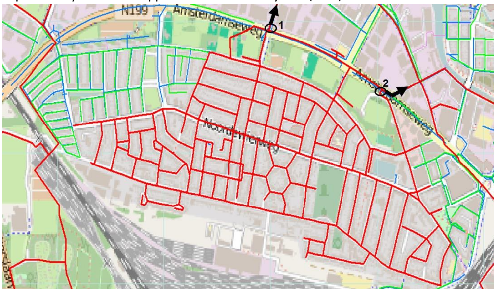
Figure 1.7: type of sewer pipes in the Soesterkwartier. Red = combined; green = dry weather system; blue = rain water system (Kikker, 2016). 1) internal overflow; 2) sewer pumping station.
