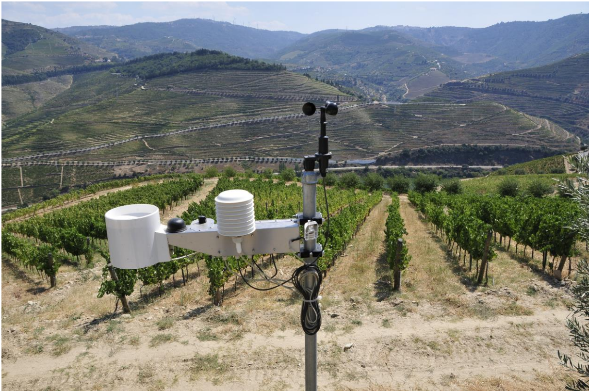
Figure 19. Meteorological instruments in the Douro region that are used for weather forecast, which is required to find the best times to apply pesticides on the vineyards to reduce the overall pesticide use. Also illustrated on this image are vertical plantations on the foreground and horizontal plantations on the other side of the river, on the background. Authors' own image.
