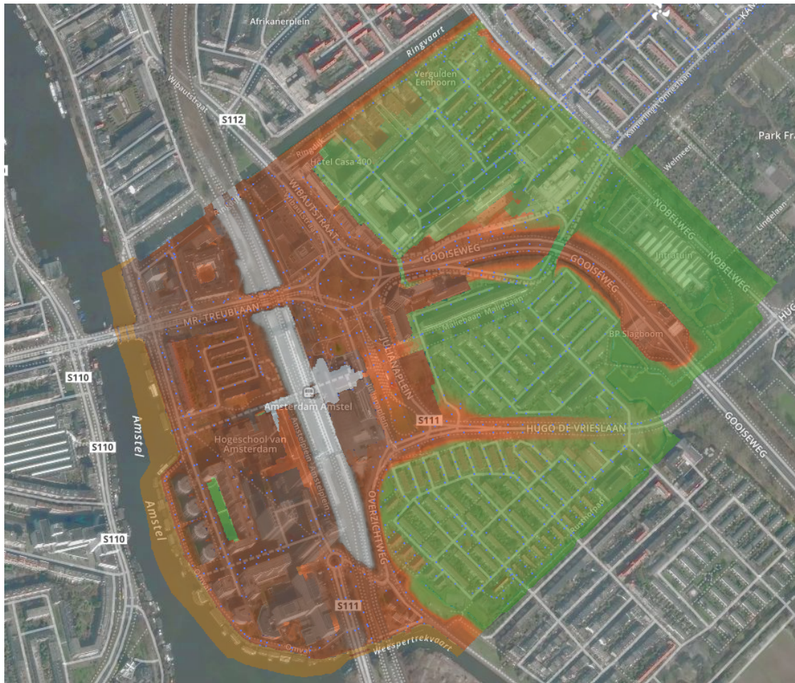
FIGURE 4.14: The area used in the 3Di modelling. The area is a part of Amsterdam, centered around the trainstation Amsterdam Amstel. The DEM is shown in red and green.
