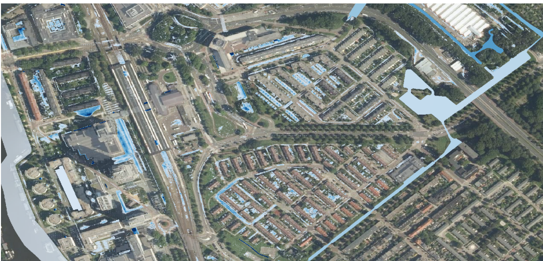
FIGURE 4.19: Inundation depths at t=157 minutes after start event (maximum levels).
