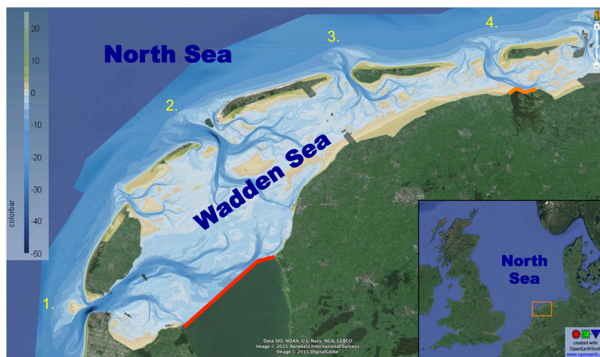
Figure 1.1: Bathymetry of the western Wadden Sea combined with the satellite image of this region using Open Earth Tools. The red and orange line indicate the dikes that close the Zuiderzee and Lauwerzee. The numbers 1 to 4 indicate the Texel Inlet, Vlie Inlet, Ameland Inlet and the Zoutkamperlaag Inlet, respectively. The bathymetry was measured in the period 2006 to 2012 by Rijkswaterstaat. Reprint from Ridderinkhof [2016]
