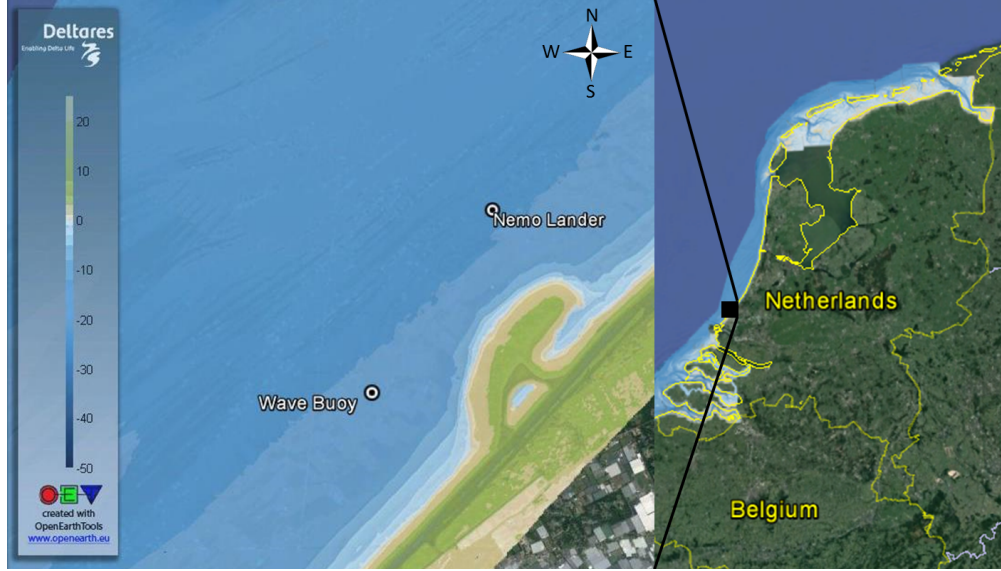
Figure 3.1: Google earth map of the measuring site. The bottom topography is added using OpenEarthTools in combination with the vaklodging of 2011. The surface elevation measurements were obtained at the dot labelled Wave Buoy and the bottom velocity measurements were obtained at the dot labelled Nemo Lander.
