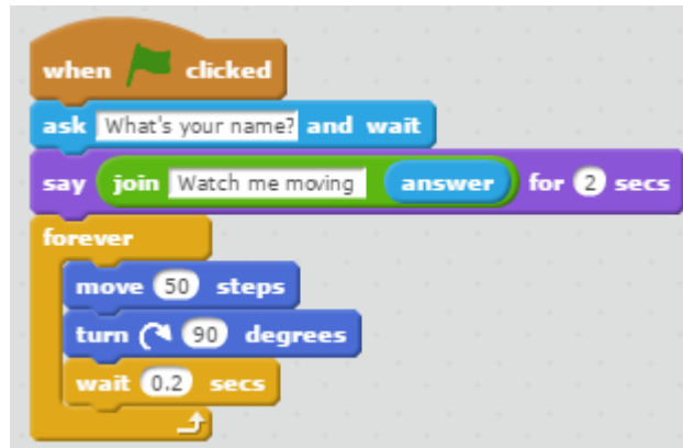
Figure 1: An example of Scratch code: the cat asks for your name, says something with your name, and then walks in the shape of a square.
