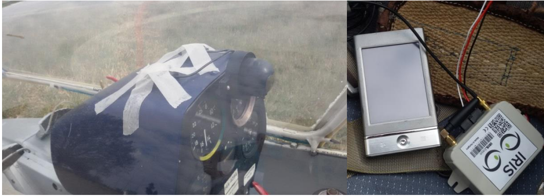
Figure 14: IRIS device external GNSS antenna (left) and IRIS device next to navigational PDA
