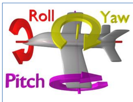
Figure 1: Roll, pitch and yaw of an aircraft (Wikipedia/Flight dynamics, 2014)
