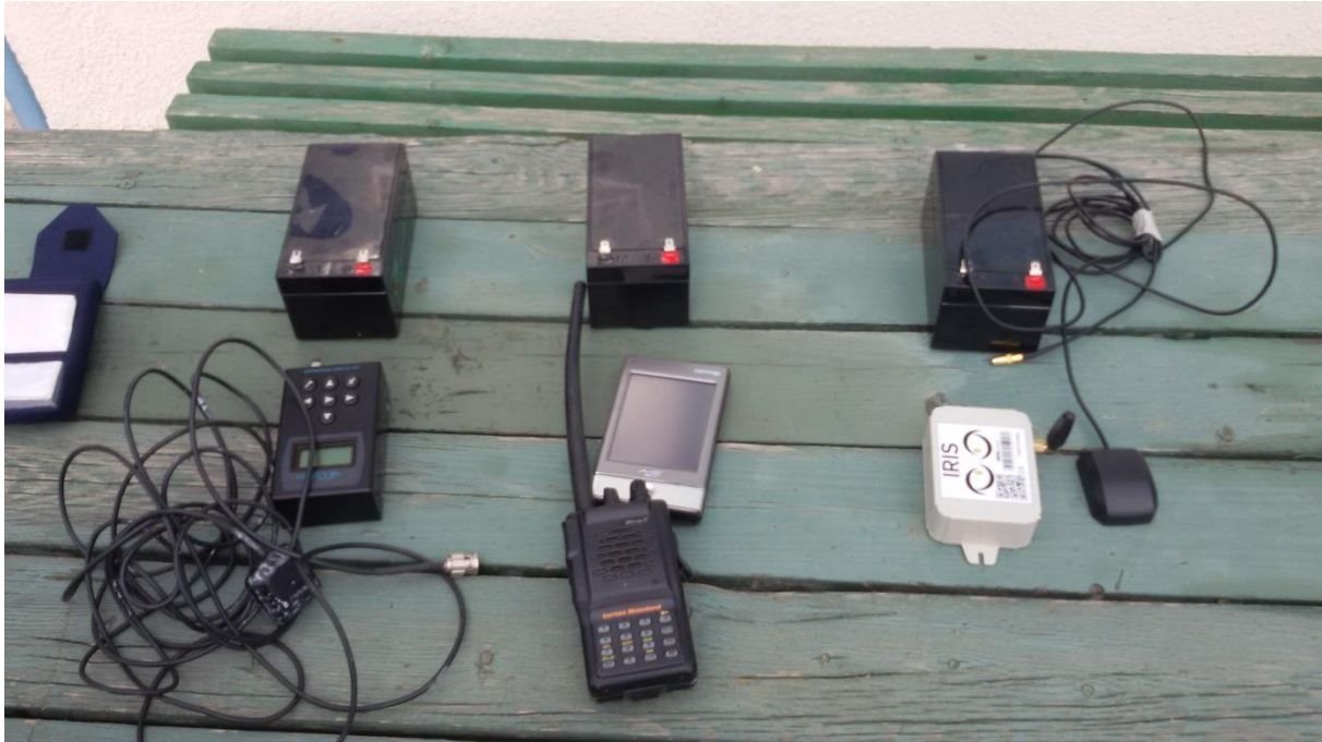
Figure 13: Flight recorder (left), radio and navigational PDA (middle) and IRIS (right) with extra batteries
