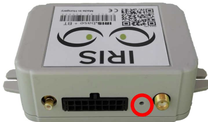
Figure 28: IRIS device, reset button is highlighted in red circle
