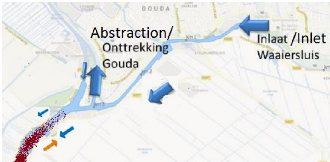
Figure 2.11. Freshwater buffer on the Hollandse IJssel for the KWA+. Water is supplied from HDSR through the Waaiersluis. By limiting the water abstraction at Gouda a “freshwater buffer” is created (modified from HydroLogic, 2014).
