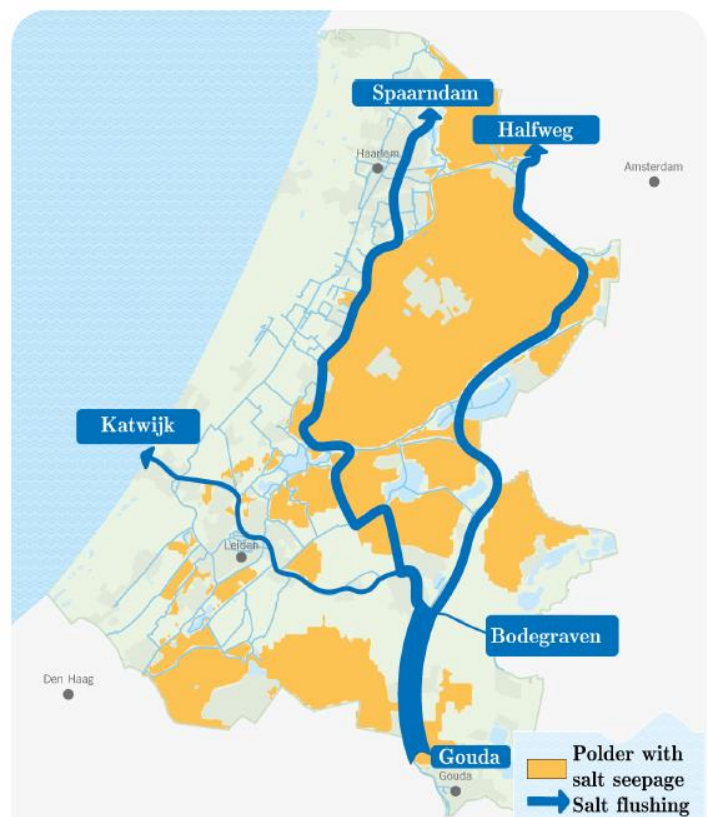
Figure 2.1. Schematization of the Rijnland boezem system during flushing and locations of polders with salt seepage. (Rijnland, 2009).
