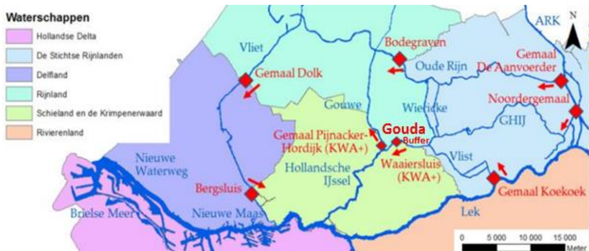
Figure 2.10. Route of the KWA(+). The Red arrows indicate the routes by which freshwater is supplied to Rijnland when the KWA(+) is active. During regular situations freshwater is let in at Gouda (Modified from Hydrologic, 2015a).
