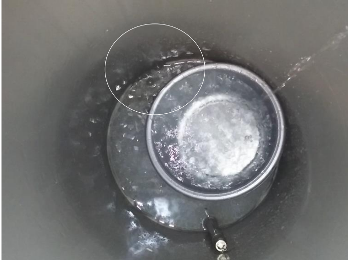
Figure 4-5 Experiment V, at the top of the column air bubbles erupted (in the white circle) during the early stages of the experiment, when the ponding layer had not reached its full height yet. The water was supplied by a tap at a height of about 60.0 cm above the soil surface, therefore a grey container was placed, to prevent the falling water from disturbing the soil surface.
