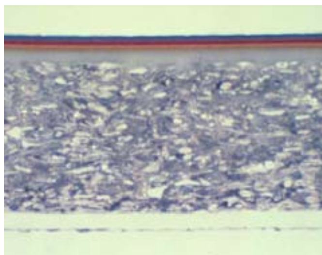
Figure 6: Cross section of photographic paper.
