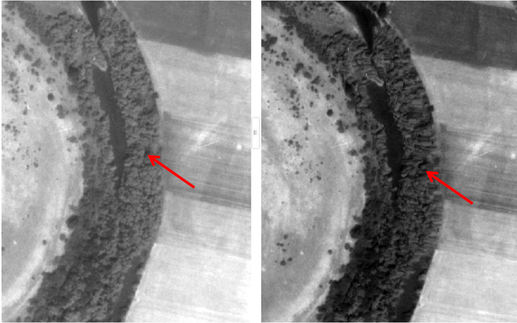
Figure 2.5: Distortions in trees caused by resampling are seen in the dark bend of trees indicated with a red arrow
