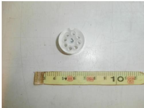
**Figure C-1.** Araldite DBF epoxy cylinder block (stub) of one inch diameter with eight drilled holes (4.5 mm diameter) in which sample is put.
