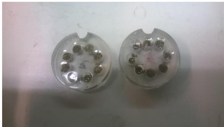
**Figure C-6.** Stub with holes filled with matrix sample and Araldite 20-20.
