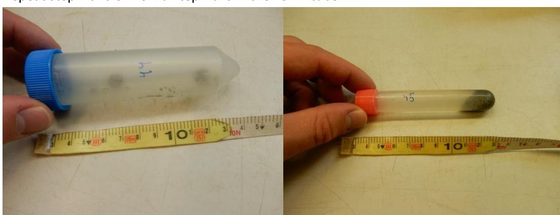
**Figure C-3. a.** 15 ml tube filled with isolated tephra. **b.** residue of the matrix sample.
