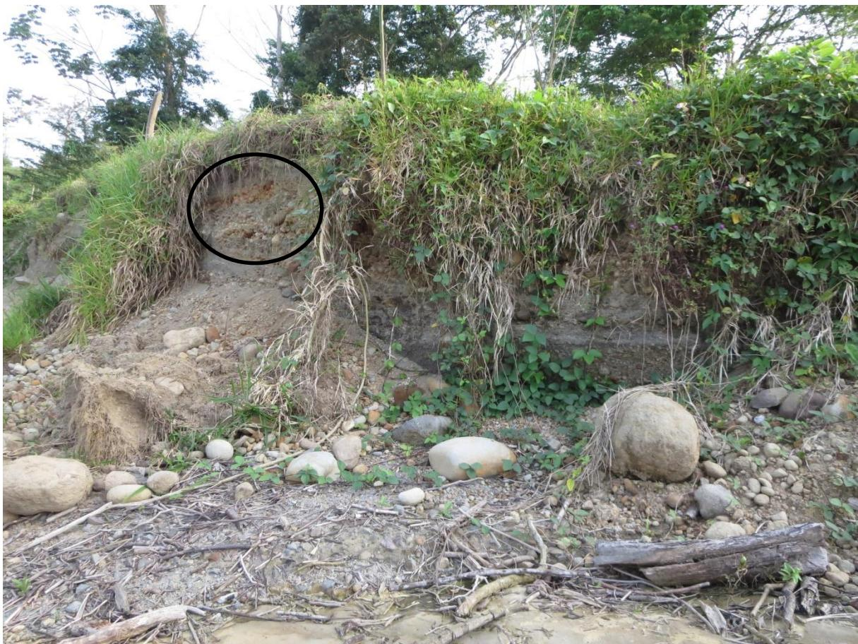
**Figure A-18.** 2m terrace close to the river overgrown with vegetation, but little weathering. Circle shows fresh surface from which samples were taken.
