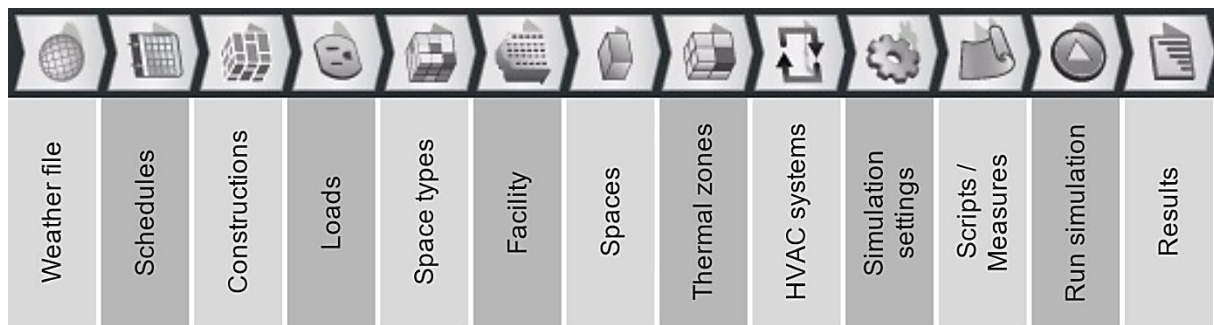
Figure 5 OpenStudio workflow based on the actual structure of the software (OpenStudio, 2015b)
